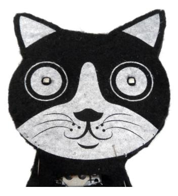
Before you start sewing you will need to cut a small hole in the centre of each eye so that the LEDs can be seen.
