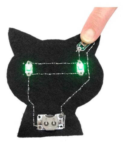
It is important to make sure the circuit works before it is sewn into the cat. This is because once it is sewn into place it will be difficult to correct any faults.
