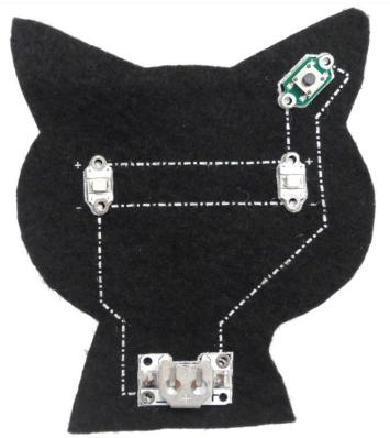
Now it is time to sew the electronic parts on to the piece of felt shown to the left. It is important to ensure that the coin cell holder and LEDs are in the correct orientation otherwise the circuit might not work.
