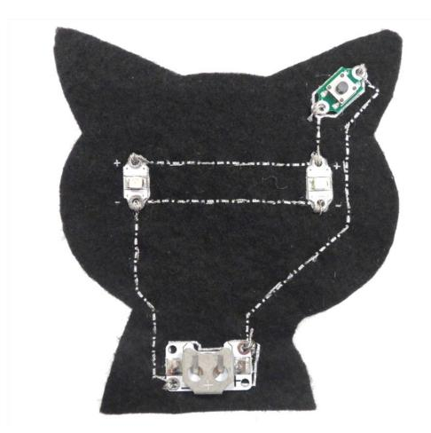
Once you are happy sewing with the conductive thread it is time to sew all of the parts in place. This needs to be done in three stages.
