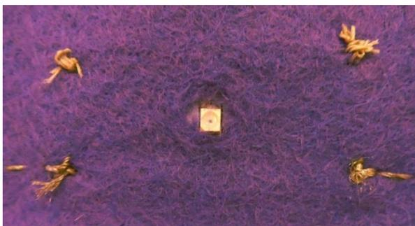
With the board sewn securely down, feel where the phototransistor is and cut a small rectangular hole for it to stick out through, this is best done with a pair of scissors. Make sure the whole surface of the phototransistor is exposed.
