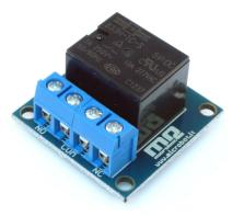
This *Relay Module* is a module designed to allow you to control a single relay in a very simple and intuitive manner. Being compatible with Arduino, the most immediate way to use it is to connect it to an Arduino board using flexible jumpers.
