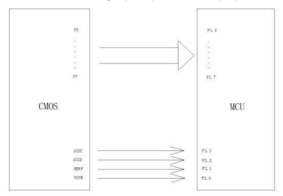
User according to the figure above simply the fifo read data timing control pin, data can be read directly by the MCU IO port data into memory or sent to the screen memory display can be operated by low-speed MCU control, and simple processing of the data, such as black and white identification.
