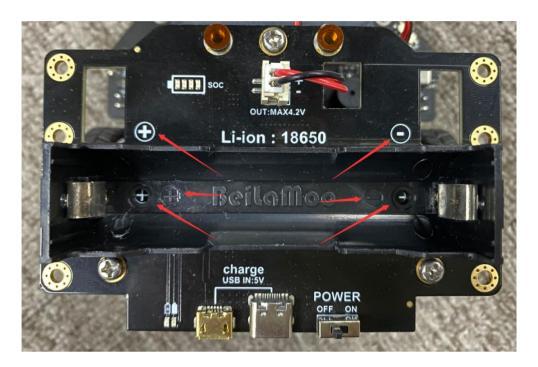
Before installation, please ensure that the "POWER" switch is turned to the "OFF" side.
