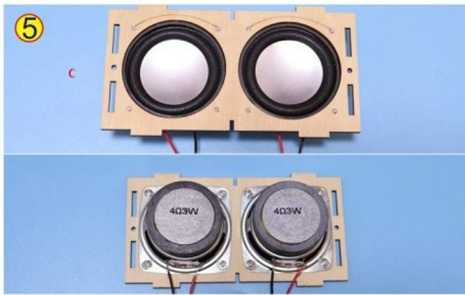
5.Eight short screws to secure the horn
