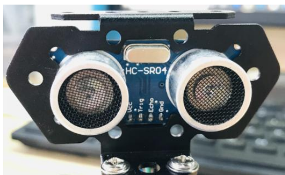
3. Install the ultrasonic sensor and connect it to the corresponding interface with 4P wire
