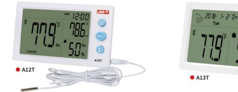
A12T/13T measures real-time temperature and humidity and display readings on a large screen. These can be used for both indoor and outdoor measurements. A12T has an additional external sensor probe for measuring temperatures of two locations. Both of these meters have alarm clock and 12/24 time mode. A12T displays comfort rating based on the combination of temperature and humidity. Hanging hole and stand are available for wall or table mount.
