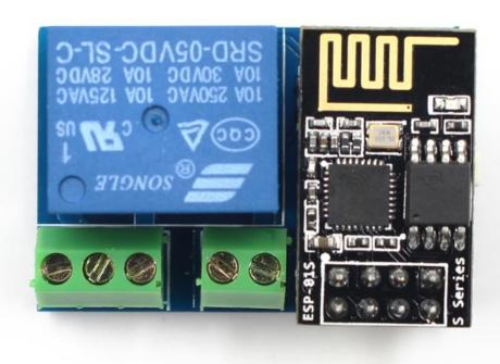
2) Power supply Connect a DC 5V power to the GND and VCC.
