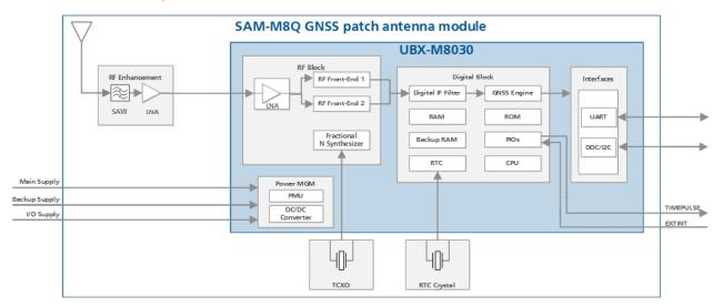
Figure 1: SAM-M8Q block diagram
