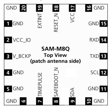
Figure 2: Pin assignment
