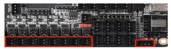
All of the fan outputs and the proximity sensor input can individually have the voltage supplied by their pin header selected by configuring the jumpers associated with each header.
