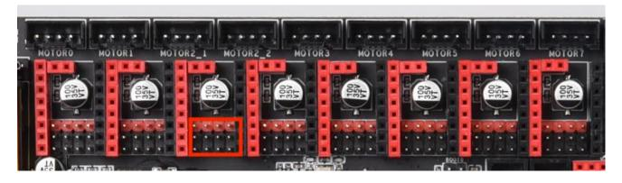
In the above image the red rectangle isolates one group of driver pins. For the purpose of running the drivers in step/dir mode the pinout can be described as per the table below (note that this is not the actual pinout but rather a simplification for step/dir mode).
