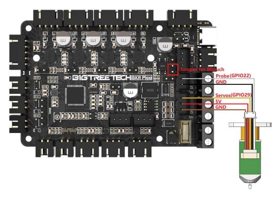
6. Connection with Proximity switch, Select the type of proximity switch as PNP or NPN by jumper  $\frac{1}{2}$
