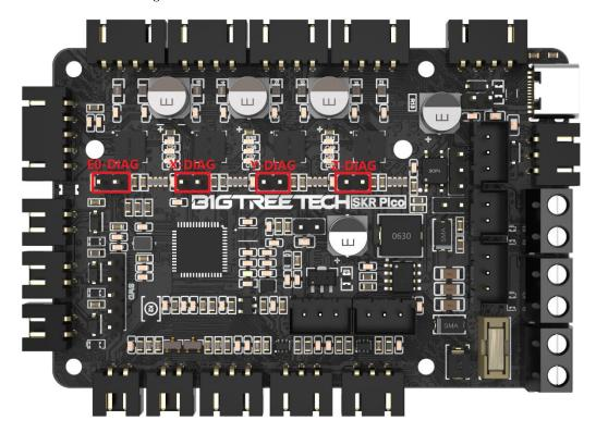
The jump caps are connected to corresponding axis as show NOTE: If you select this function, you cannot use external ENDSTOP!!!
