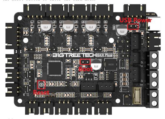
(2) Connect USB-C to computer, then you will see a USB flash drive named RPI-PR2, copy compiled klipper uf2 file to the USB flash drive, the motherboard will automatically reboot and update the firmware, the computer will re-identify this USB flash drive means the firmware update is complete, unplug the jump cap and click the Reset button to enter normal working mode.
