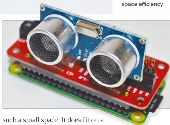
Above An ultrasonic sensor can plug straight into the board if you want to keep things compact
