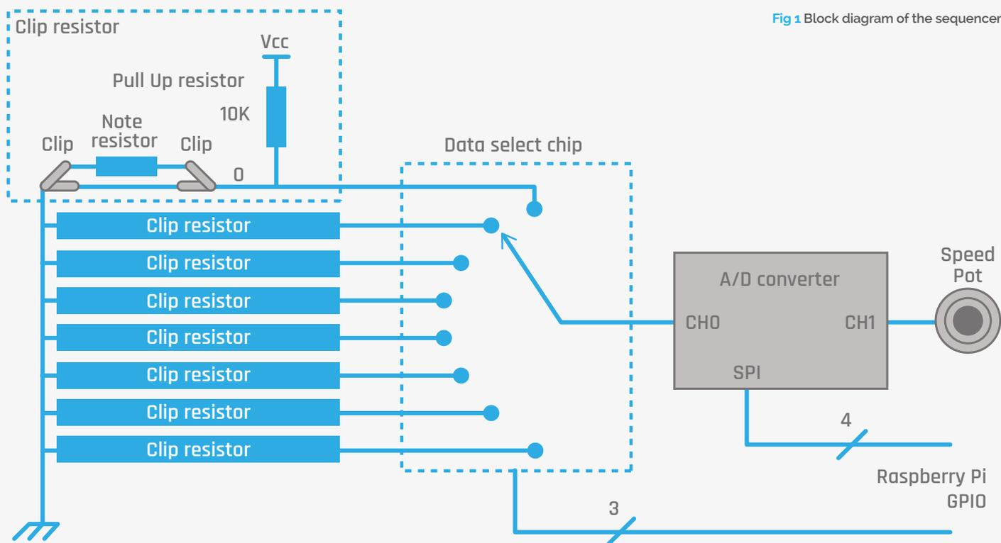
Fig 1 Block diagram of the sequencer
