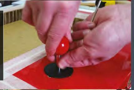
The controls are connected to an Arduino Leonardo, which translates the movement to keyboard commands and sends them to the Raspberry Pi
