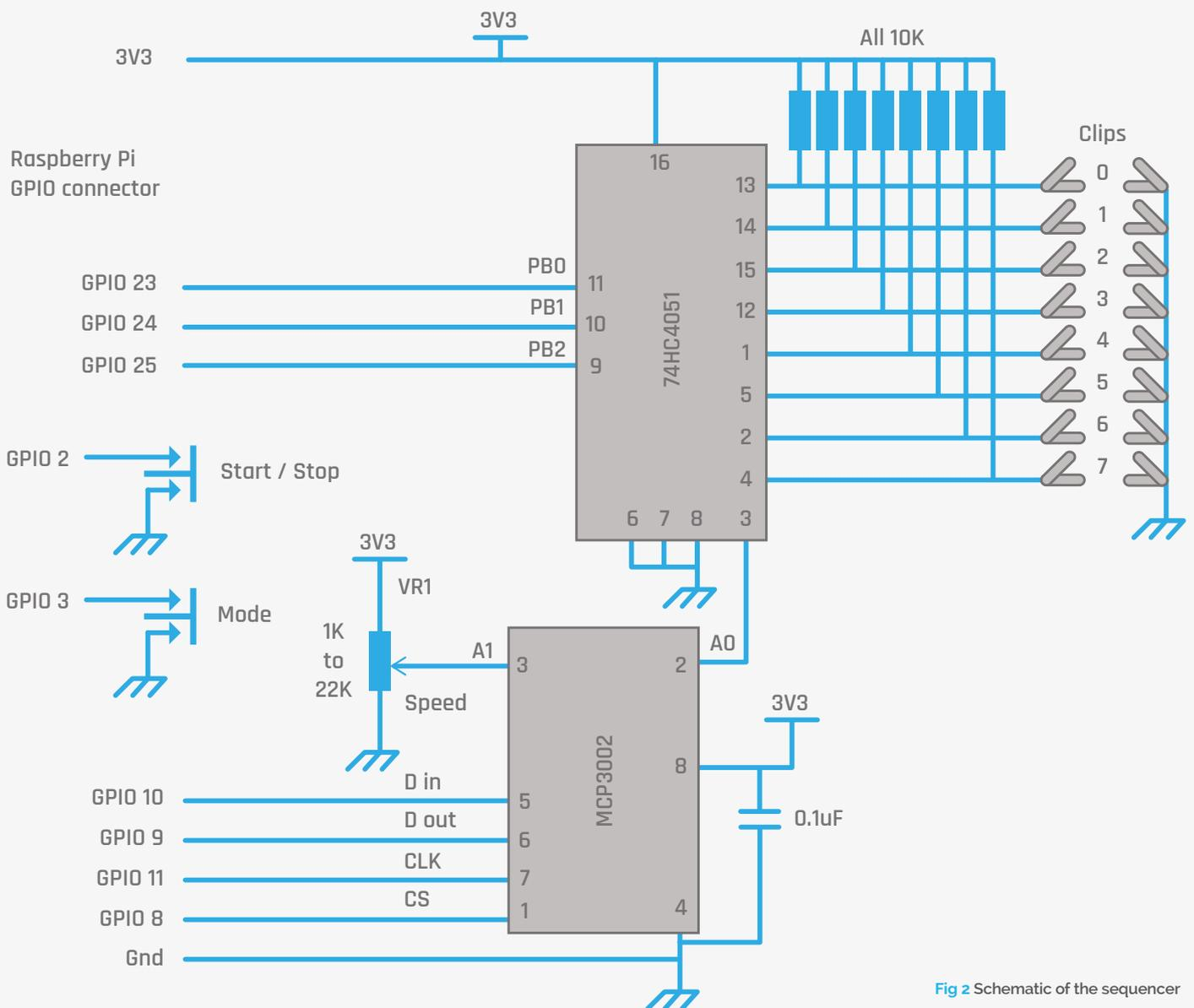
Fig 2 Schematic of the sequencer
