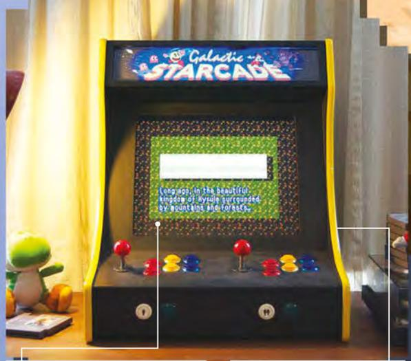
A 19-inch LCD TFT monitor with built-in speakers provides both video and audio output
