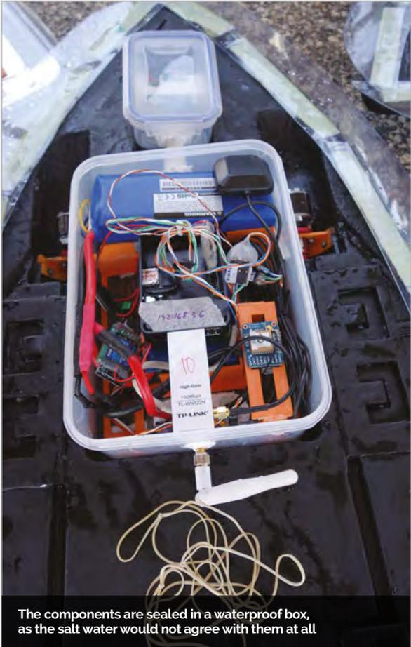
The components are sealed in a waterproof box, as the salt water would not agree with them at all
