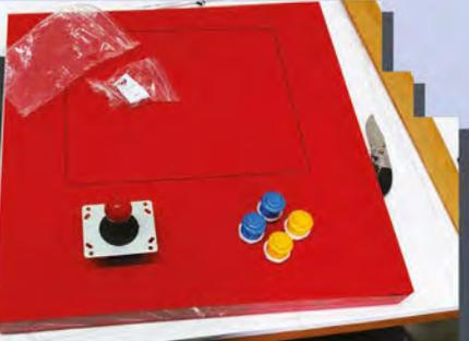
Holes drilled into the surface house the joystick and buttons. The controls are inserted from underneath
