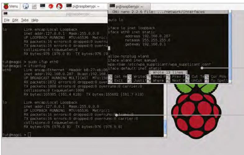
`/etc/network/interfaces` contains an entry telling the Pi to use DHCP to allocate an address. Change it to static, and give your board a permanent address
