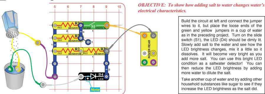
Build the circuit at left and connect the jumper wires to it, but place the loose ends of the green and yellow jumpers in a cup of water as in the preceding project. Turn on the slide switch (S1), the LED (D4) should be dimly lit. Slowly add salt to the water and see how the LED brightness changes, mix it a little so it dissolves. It will become very bright as you add more salt. You can use this bright LED condition as a saltwater detector! You can then reduce the LED brightness by adding
