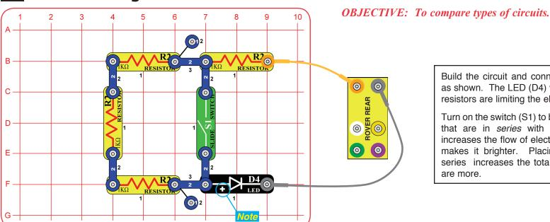
Build the circuit and connect the jumper wires as shown. The LED (D4) will be on but the four resistors are limiting the electricity through it.
