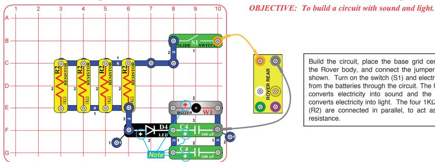
Build the circuit, place the base grid centered on the Rover body, and connect the jumper wires as shown. Turn on the switch (S1) and electricity flows from the batteries through the circuit. The horn (W1) converts electricity into sound and the LED (D4) converts electricity into light. The four 1K $\Omega$  resistors (R2) are connected in parallel, to act as a  $250\Omega$ resistance.
