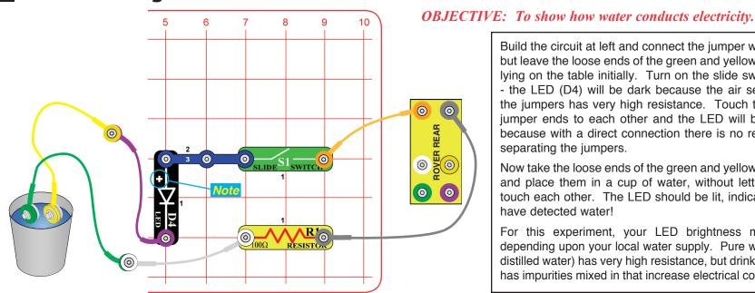
Build the circuit at left and connect the jumper wires to it. but leave the loose ends of the green and yellow jumpers lying on the table initially. Turn on the slide switch (S1) - the LED (D4) will be dark because the air separating the jumpers has very high resistance. Touch the loose jumper ends to each other and the LED will be bright, because with a direct connection there is no resistance separating the jumpers.
