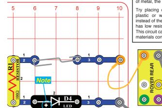
Build the circuit, place the base grid centered on the Rover body, and connect the jumper wires as shown. To complete the circuit, place a paperclip across the snaps as shown in the picture. If the paperclip is made of metal, the LED (D4) will be bright.
