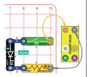
Build the circuit, place the base grid centered on the Rover body, and connect the jumper wires as shown. When you close the slide switch (S1), electricity flows from the batteries through the switch (S1), the LED (D4), the resistor (R1), and back to the battery.
