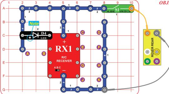
Build the circuit as shown. Be sure you have the A-B-C switches on the remote control and R/C receiver (RX1) set to the same channel, have turned on the remote control, and are not being interfered with by other remote control transmitters. Turn on the slide switch (S1), then press the left button on the remote control to turn on the LED (D4).
