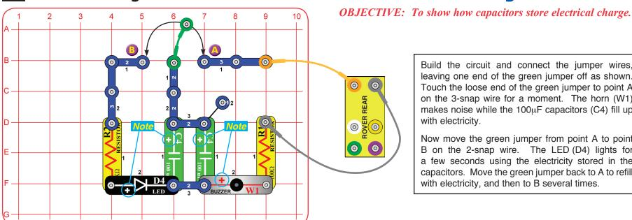
Build the circuit and connect the jumper wires, leaving one end of the green jumper off as shown. Touch the loose end of the green jumper to point A on the 3-snap wire for a moment. The horn (W1) makes noise while the 100µF capacitors (C4) fill up with electricity.
