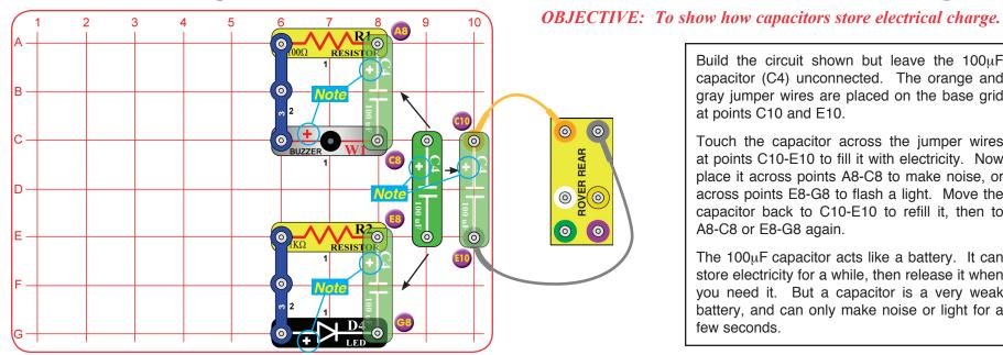
Build the circuit shown but leave the 100µF capacitor (C4) unconnected. The orange and gray jumper wires are placed on the base grid at points C10 and E10.
