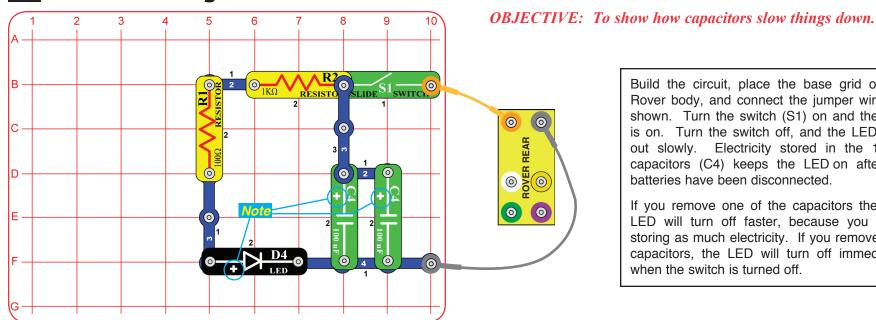
Build the circuit, place the base grid on the Rover body, and connect the jumper wires as shown. Turn the switch (S1) on and the LED is on. Turn the switch off, and the LED goes out slowly. Electricity stored in the 100μF capacitors (C4) keeps the LED on after the batteries have been disconnected.
