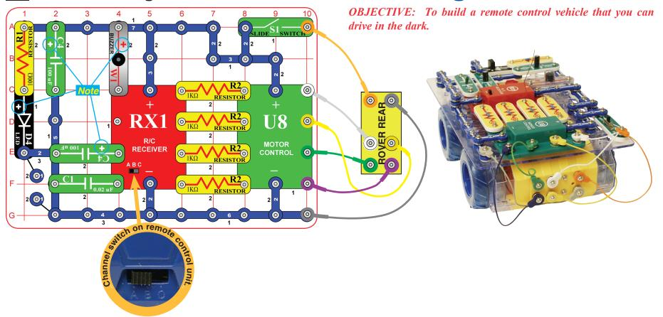
The Snap Circuits® Kit uses electronic blocks that snap onto a clear plastic base grid to build different circuits. These blocks have different colors and numbers on them so that you can easily identify them.
