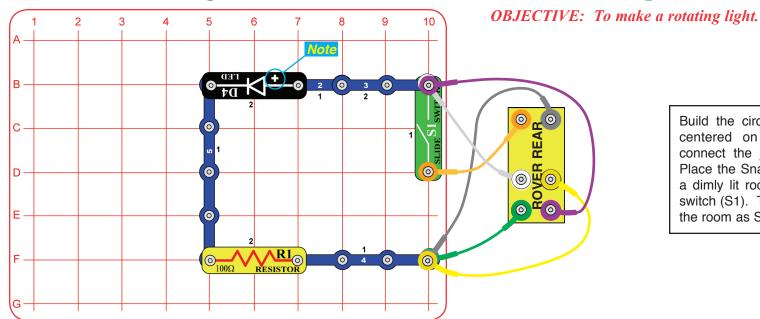
Build the circuit, place the base grid centered on the Rover body, and connect the jumper wires as shown. Place the Snap Rover in the middle of a dimly lit room and turn on the slide switch (S1). The light will shine around the room as Snap Rover spins.
