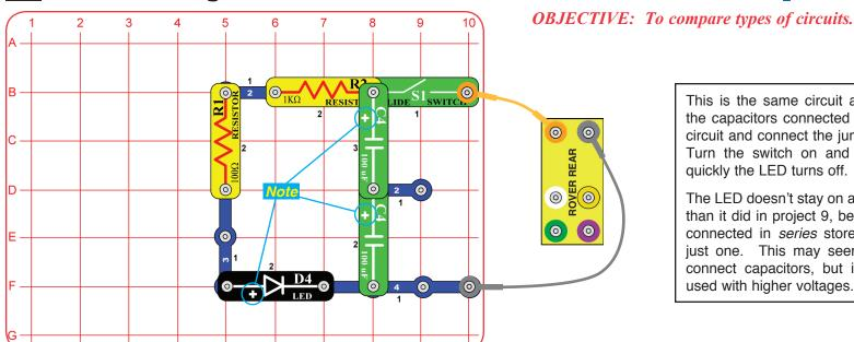
This is the same circuit as project 9, but with the capacitors connected differently. Build the circuit and connect the jumper wires as shown. Turn the switch on and off, and watch how quickly the LED turns off.
