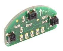
Sensor output: The sensor output voltage changes from the supply voltage to OV as the sensors pass over light and dark surfaces. Different surfaces will reflect different amounts. A typical light surface will give a value of 0.5V for example. A typical dark surface will give a value of 2.5V (assuming a 3V VCC). The value in a program will depend on the processors ADC range and width.
