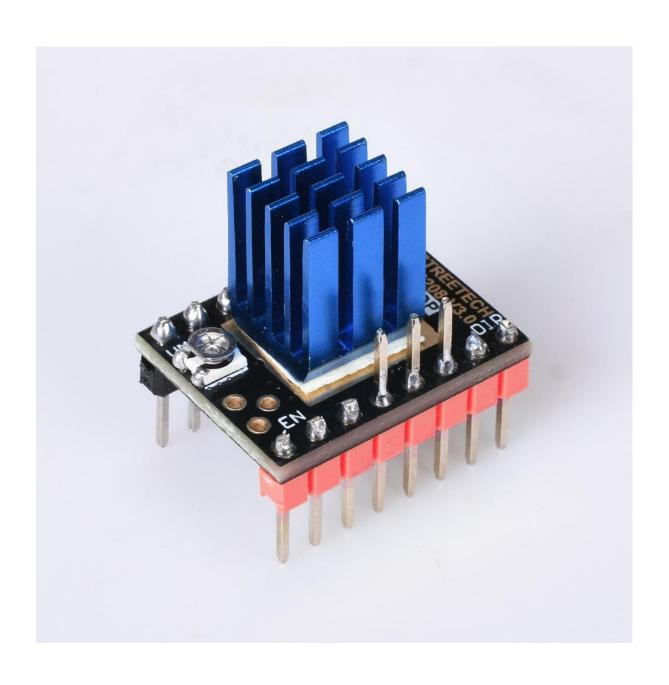
TMC2208 V3.0 single-axis stepper motor drive chip, power tube built-in drive current 1.4A peak current 2A, voltage range 4.75V-36V, 256 subdivision; with patented technology spreadCycle ™ high chopper frequency, dcStep ™, stallGuard2 ™ stall detection technology, CoolStep ™ current dynamic adjustment technology, can save 70% of the energy, StealthChop mute technology.Support Single Wire UART for advanced configuration options.Integrated Pulse Generator for standalone motion.
