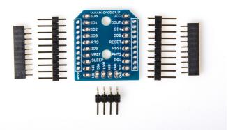
The XBee to DIP Adapter is a brakout board that allows the use of the XBee and the XBee PRO wireless modules. This board breaks out all 20 pins of an XBee module to a 0.1" (2,54mm) standard spacing dual row header. The spacing between these two headers is 0,6" (15,24mm) making this adapter DIP friendly; in this way the adapter can be used with common IC sockets, with prototyping boards and also with breadboards.
