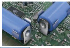
MATERIAL: Spring Steel Tin Nickel Plate
